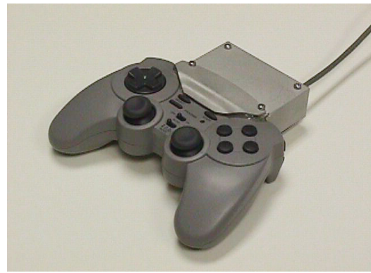
Figure 6. Videogame controller. We use a retrofitted off-the-shelf video game controller for high level control of gaze, movement and emotion.
